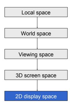
5) Collapse the box to a plane. Rasterize primitives using Z-axis information for depth-sorting and hidden-surface-removal.
