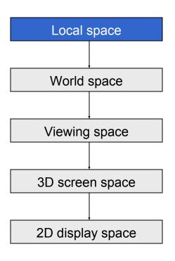
1) Geometry is defined in *local space*. The vertices and coordinates of a surface are specified relative to a local basis and origin.
