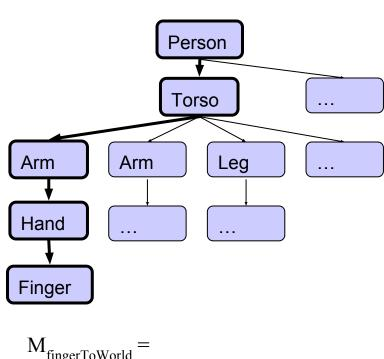
$$\begin{aligned} \mathbf{M}_{\text{fingerToWorld}} &= \\ (\mathbf{M}_{\text{person}} \bullet \mathbf{M}_{\text{torso}} \bullet \mathbf{M}_{\text{arm}} \bullet \mathbf{M}_{\text{hand}} \bullet \mathbf{M}_{\text{finger}}) \end{aligned}$$
