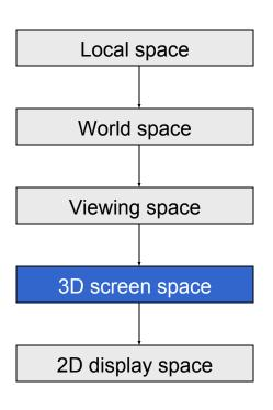
4) Perspective: Transform the viewing frustrum into an axis-aligned box with the near clip plane at z=0 and the far clip plane at z=1. Coordinates are now in 3D screen space.
