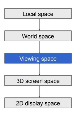
3) Rotate and translate the geometry from *world* space to *viewing* or *camera* space.
